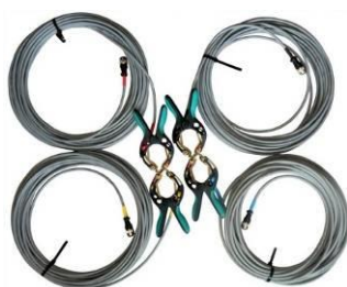
X winding test cable set
